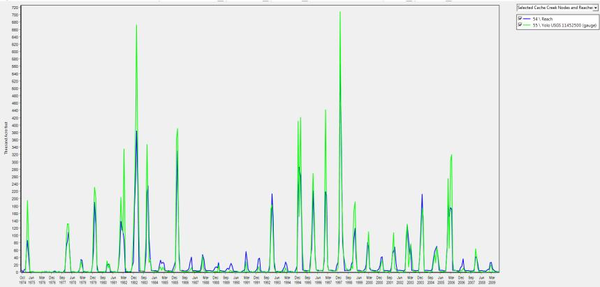
Figure B 13. Observed and modeled streamflow in Cache Creek at Yolo
