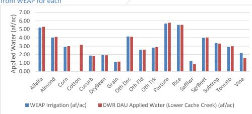
Figure B 11. Comparison of average applied water from Lower Cache Creek DAUE and average irrigation from WEAP for each
