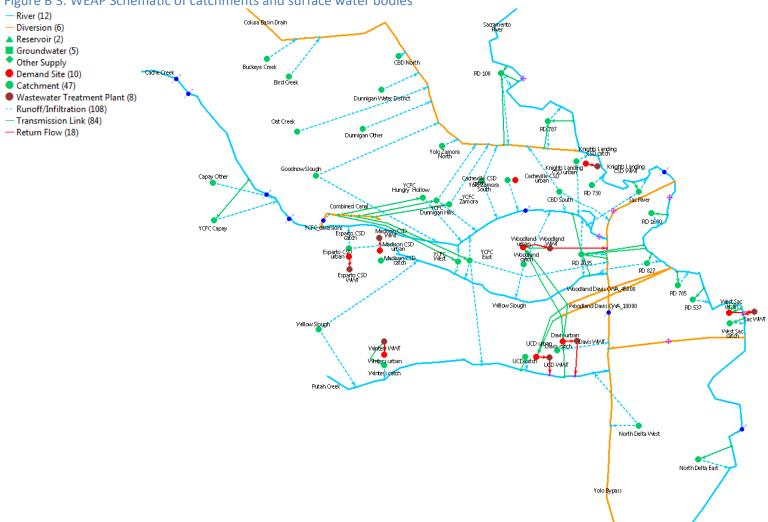
Figure B 3. WEAP Schematic of catchments and surface water bodies
