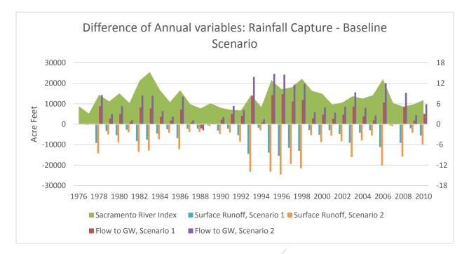
Figure 4.4 Difference of annual surface runoff and flow to groundwater between the rainfall capture and baseline scenarios.
