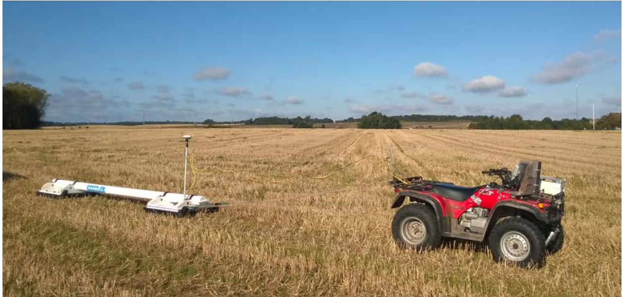
Figure B.2 - DUALEM421s sensor pulled behind ATV
