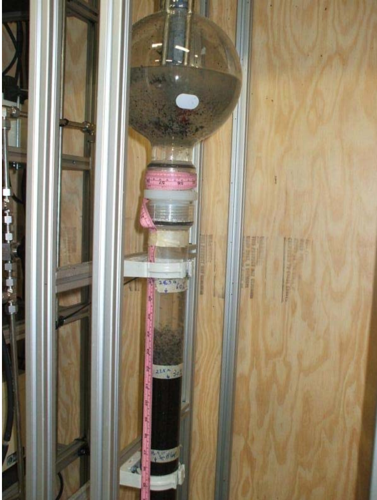
Photo #5: FBR Pilot in Operation
