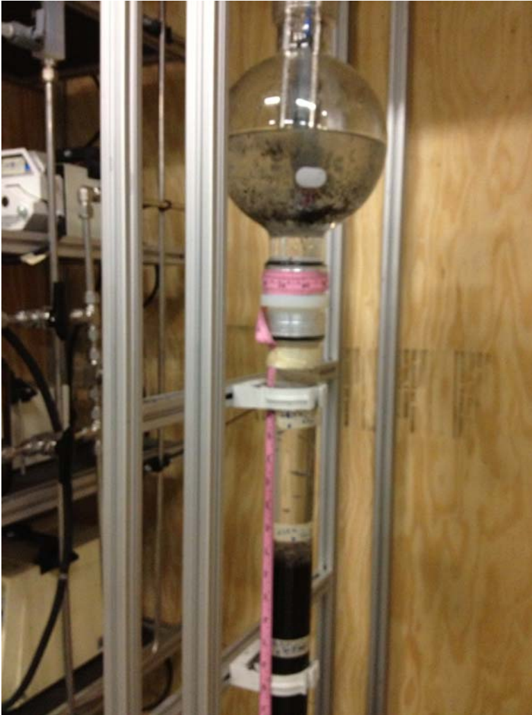
Photo #6: FBR Pilot in Operation
