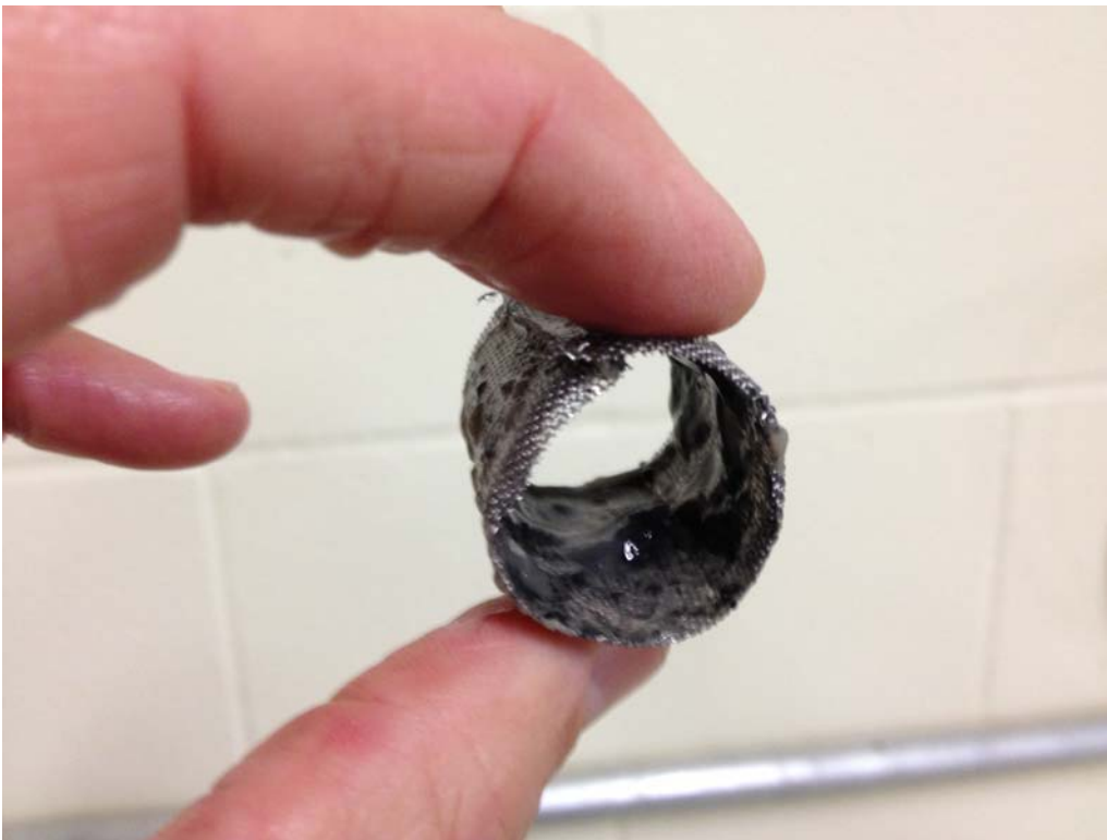
Photo #9: Clogged Basket Strainer
