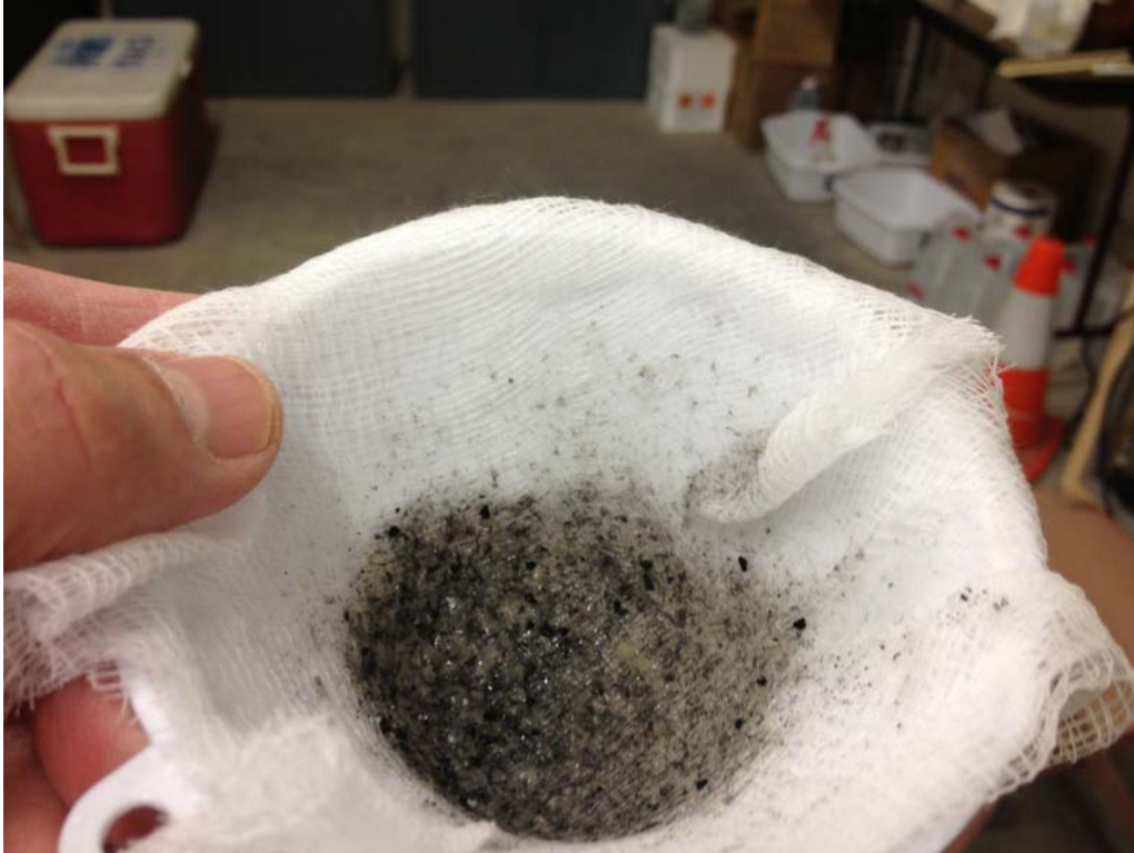
Photo #10: Filtered Biomass After Cleaning
